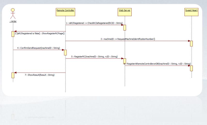
4. Register a remote controller on the DB
