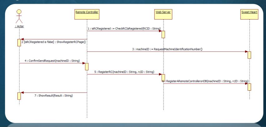
4. Register a remote controller on the DB
