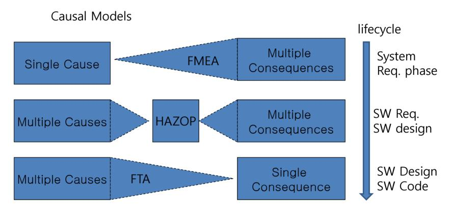
Focused HA through lifecycle Harmonized (top-down and bottom-up) HA HAZOP checklists with guidewords developed by KAERI and LLNL FTA templates for FBD program
