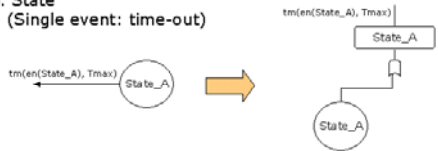
(b) Templates for transforming labeled digraph into goal-tree
