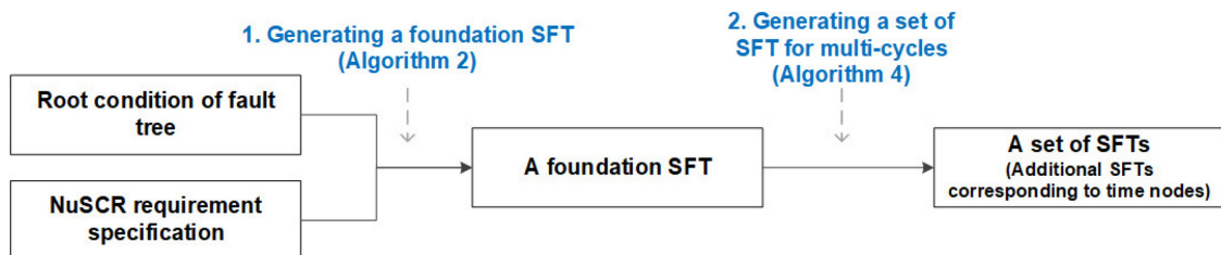
Fig. 8. A process of the SFT construction algorithm
